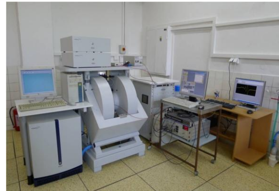
X-band EPR spectrometer (Bruker EMX, Germany)
