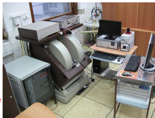
X-band EPR spectrometer (Bruker EMX, Germany)
